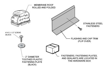
• Check the roof of the walk-in unit and remove any foreign matter. Seal all protruding rough edges and screw heads, rivets, etc. with tape or sealant. This will prevent any chance of penetrating or wearing a hole in the membrane roof cap.
