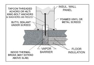
• Apply two beads of non-drying butyl sealant to the bottom side of the screeds.
