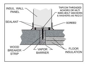
• Flat-bottom walls are available for configurations that require a metal screed, do not have an integral cove, and will be anchored by an exterior (or interior) mounting angle. Mounting angles are supplied in 10' lengths and field cut to fit the dimensions of the enclosure as necessary.
