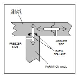
• Outdoor applications: Apply butyl tape to the partition wall anchor plate. Lock ceiling panels together and align over partition wall. Once all ceilings are assembled and aligned, attach lag bolts through the ceiling cam lock hole into the anchor plate.
