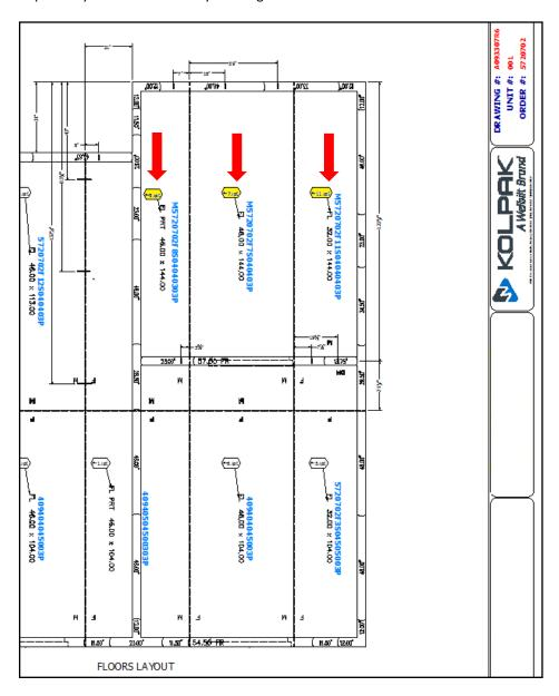
Panels are labeled with numbers corresponding to those on the assembly drawing.
